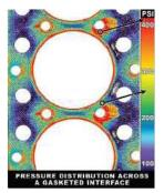
create sealing flaws. In hydraulics and pneumatics, it improves fluid power by diagnosing current and potential leakage areas in fittings, couplers and connectors.
